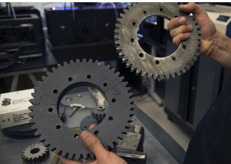
“We like Tough PLA because we can thread directly into the part and mount other components to it,” explains Mechanical Engineer, Tony Rivera. “In the time it would have taken to order a metal part and have it shipped here, we already finished the entire project.”
