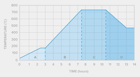
The Standard Burnout schedule is designed for compatibility with R&R Plasticast or similar investment materials. Use this schedule as a starting point and make adjustments as needed.
