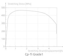
Tensile stress-strain curve
