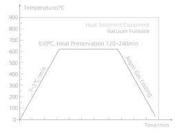
Ti-6.5Al-1Mo-1V-2Zr Process diagram of heat treatment curve
