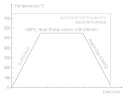
Cp-Ti Grade1 Process diagram of heat treatment curve
