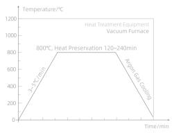
Ti-6Al-4V Grade23 Process diagram of heat treatment curve
