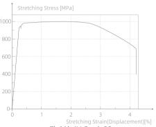
Ti-6Al-4V Grade23 Tensile stress-strain curve
