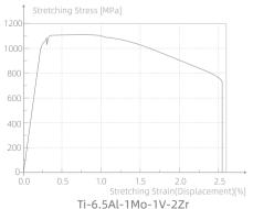
Tensile stress-strain curve
