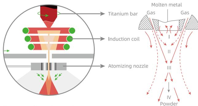
Using crucibleless electrode induction inert gas atomization technology, the powder products have characteristics of low oxygen content, high purity, high Sphercity and few satellite particles, which meets the strict requirements of additive manufacturing on powder.
